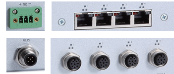
Optional M12 type for DC-in jack and LAN jack
