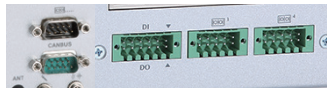
1 x DIO (TB) and 2 x COM (TB) 1 x COM (DB9) and 1 x CANbus/COM (DB9)
